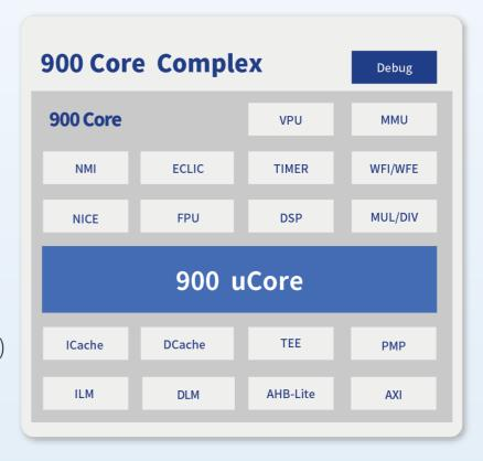
900 Series supports both instruction and data local memory (ILM/DLM) gives better real time processing capability. User can also configure instruction and data cache (I-Cache/D-Cache) to improve the performance of the overall subsystem.
